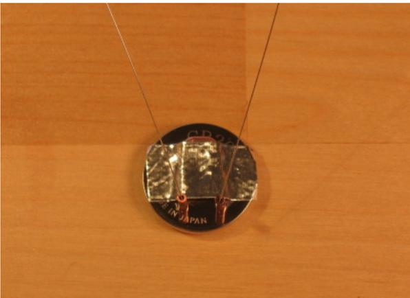
Put the antennae / battery assembly aside for now. Next, grab the remaining, smaller piece of foil tape, and peel off the backing. Pick up the LED eyes, holding on to them by one of the looped leads, and hold it upside down. Position the foil against the *twisted* LED leads, like so:
