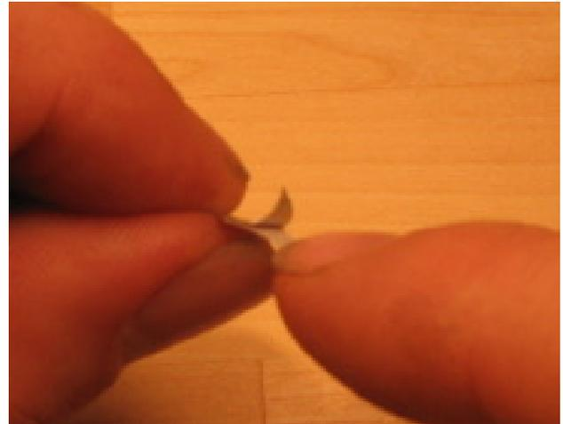
Try not to touch the sticky side, or it won't stick as well. (This foil has a special adhesive that conducts electricity, to help your Blinkybug light up).
